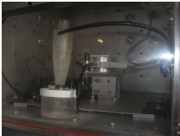
Figure 4. Honeybee's pneumatic transfer system proof of concept, in a vacuum chamber.
