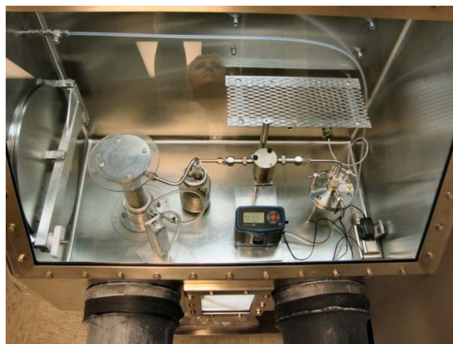
Figure 3. Pneumatic particle size separation down to 1.7 micrometers has been achieved in the laboratory.
